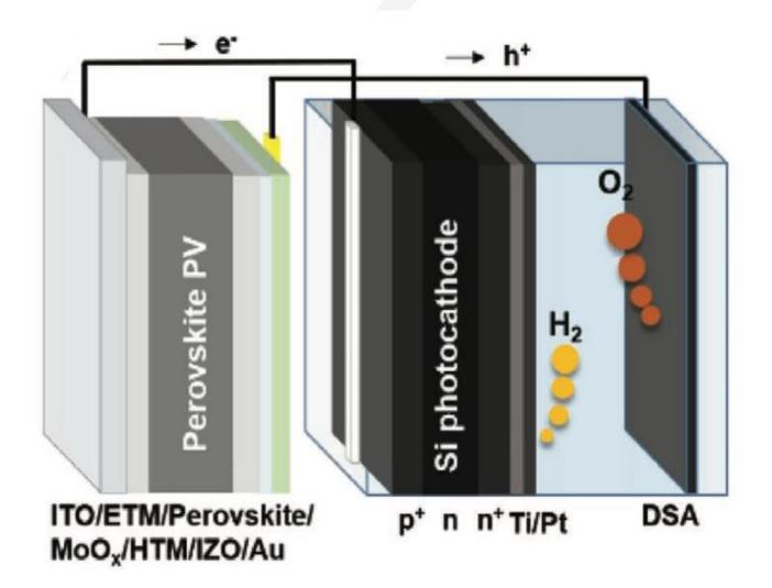
Australian researchers have claimed a new world efficiency record of 17.6% for solar panels that can directly split water using sunlight. They use a photoelectrochemical (PEC) solar-to-hydrogen (STH).
