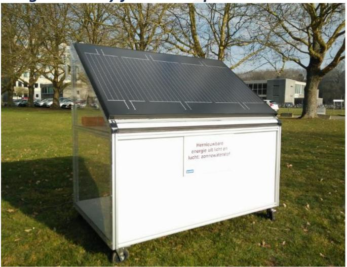
Bioscience engineers from KU Leuven have designed a hydrogen panel that converts 15 per cent of the sunlight straight into hydrogen gas – a world record.
